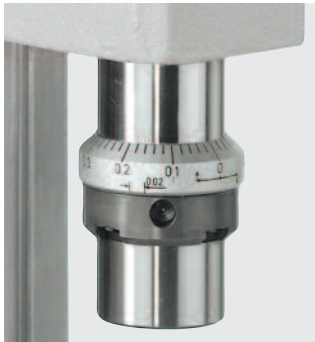
Fine adjustment for press No. 33 with scale 1 division line = 0.02 mm
